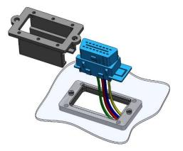
Put the OBD socket jack into the OBD-Saver housing Now mount both (housing and socket jack) onto the mounting bracket with the provided allen screws
